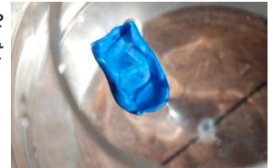
Clay in a ball shape sinks, but in a boat shape floats.
