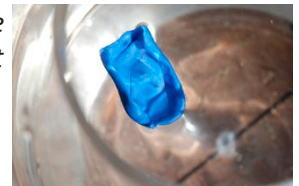
Clay in a ball shape sinks, but in a boat shape floats.
